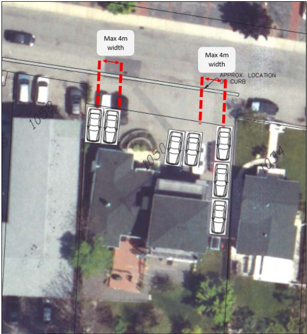
Figure 10 – Conceptual Site Plan (exact location of driveways to be determined with staff and property owner)
