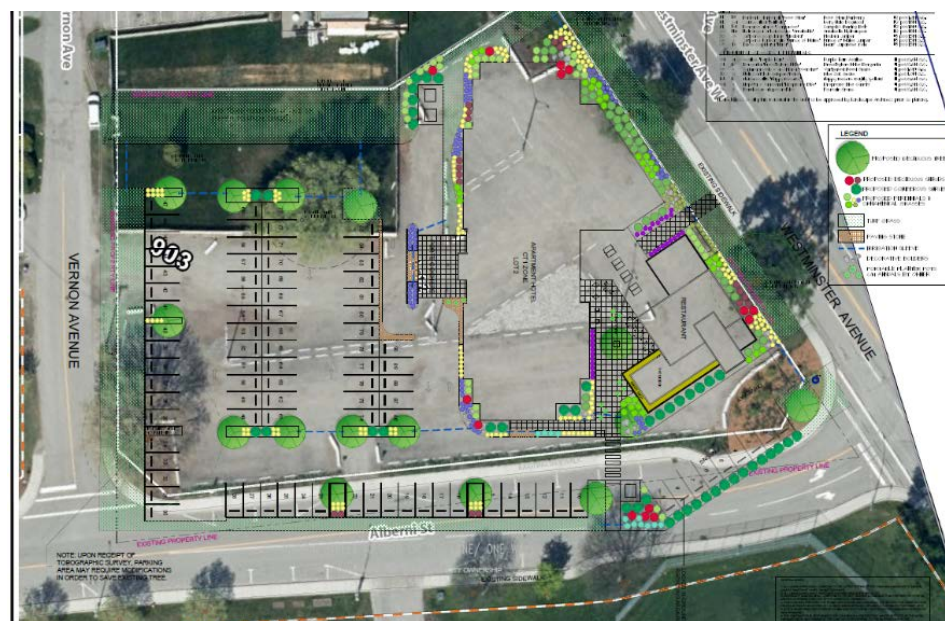
Figure 3: Site plan showing building footprint and proposed use of closed road
