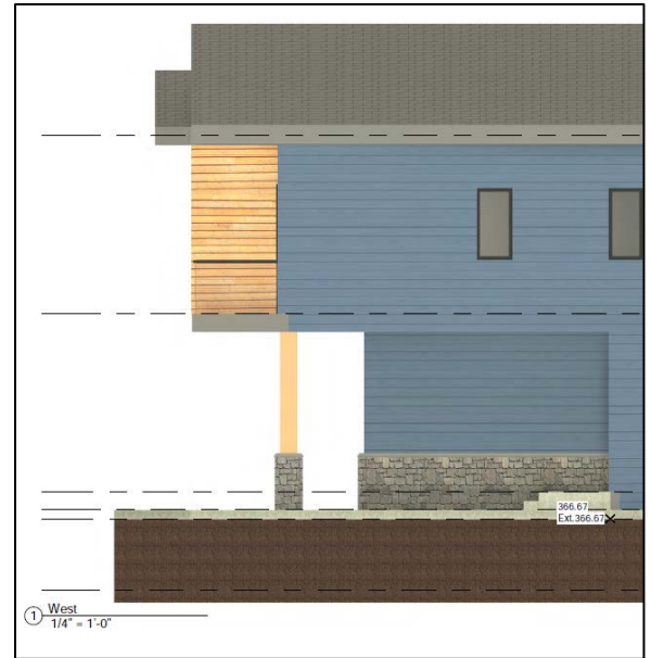
Figure 4 - Side view of proposed cantilever over driveways
