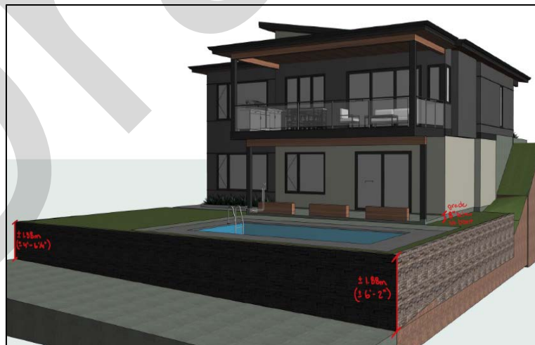
Figure 1 – Proposed retaining wall.
