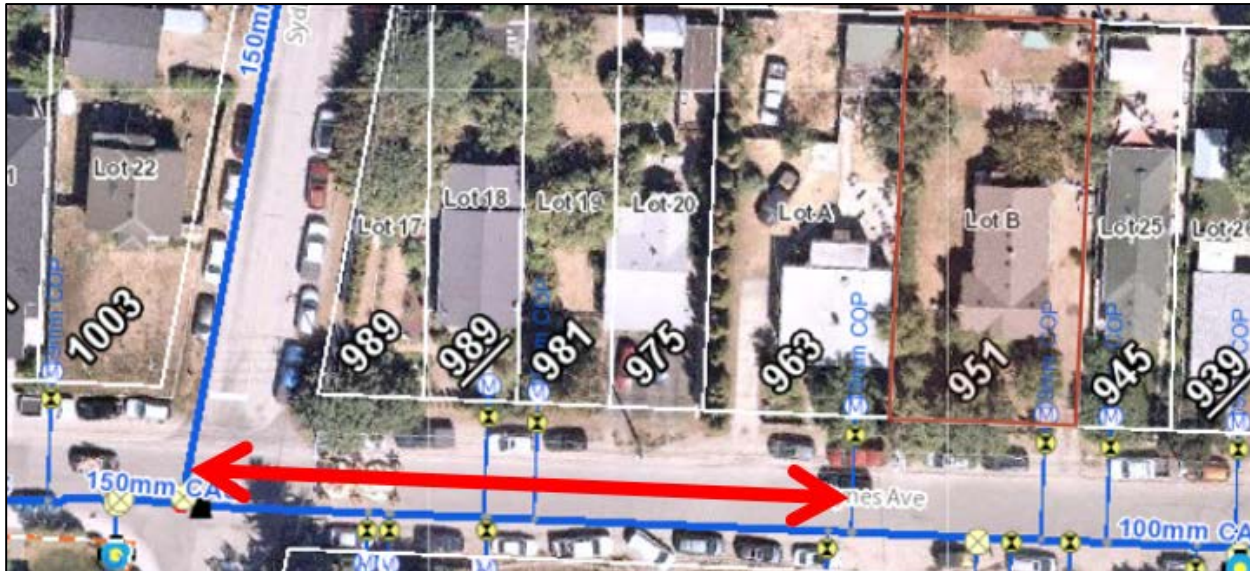
Figure 3 - Location of Water Main Requiring Upgrade
