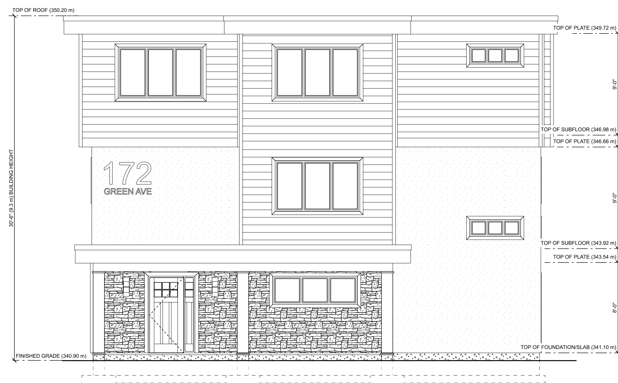
NORTH ELEVATION (FACING GREEN AVE. W.) SCALE: 3/16" = 1'-0"
