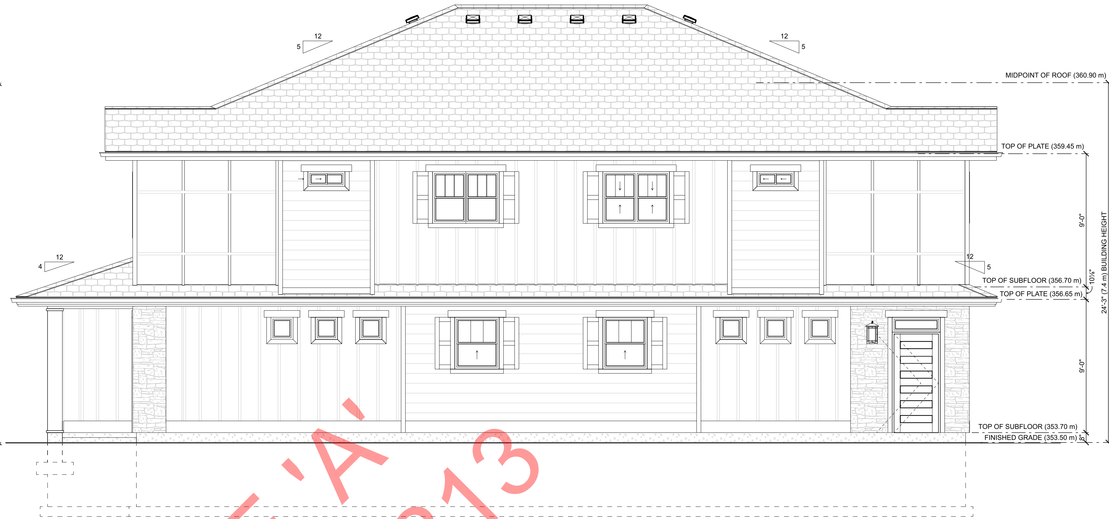
BUILDING A-RIGHT ELEVATION (FACING EAST) SCALE: 1/4" = 1'-0"
