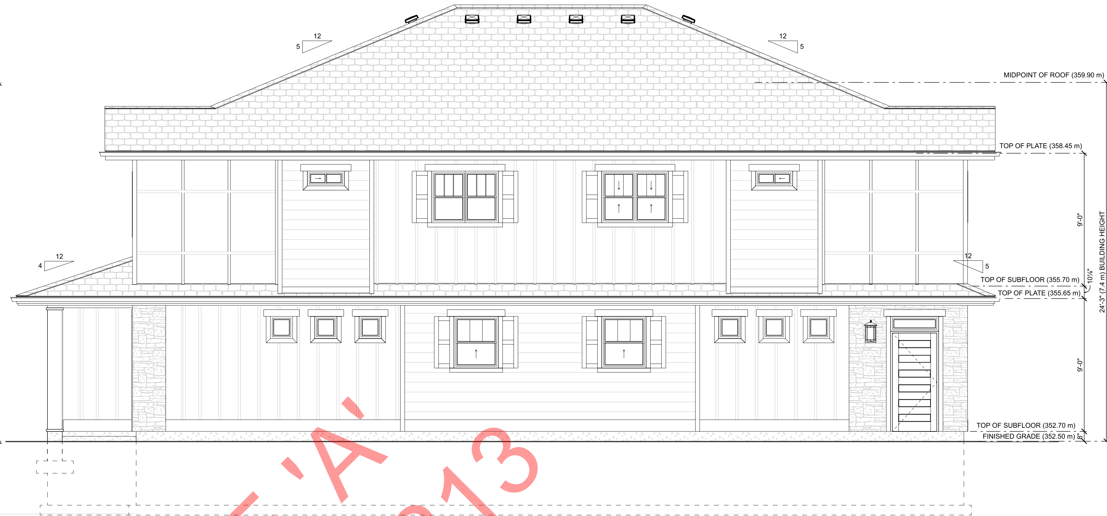
BUILDING B-RIGHT ELEVATION (FACING WEST) SCALE: 1/4" = 1'-0"
