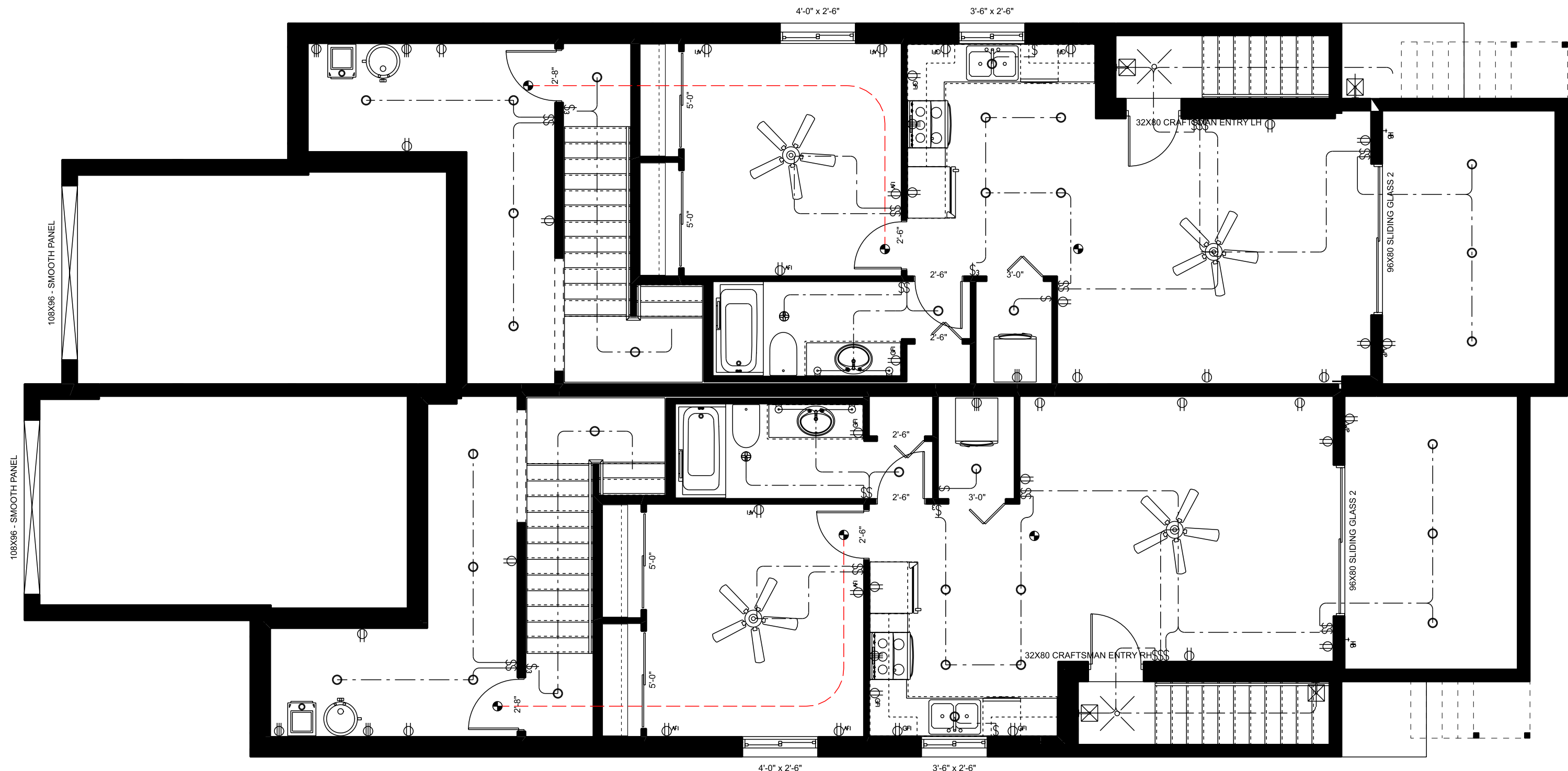
BASEMENT FLOOR ELECTRICAL PLAN SCALE: 3/16" = 1'-0"
