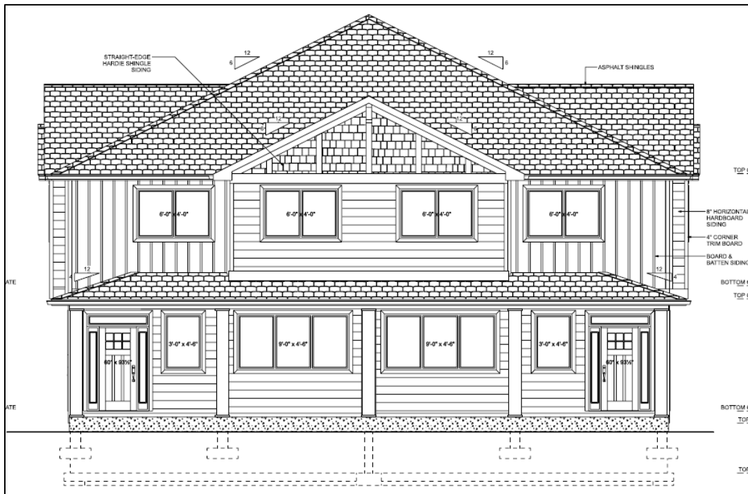
Figure 10: South Elevation of four-unit townhouse (from Calgary Avenue)
