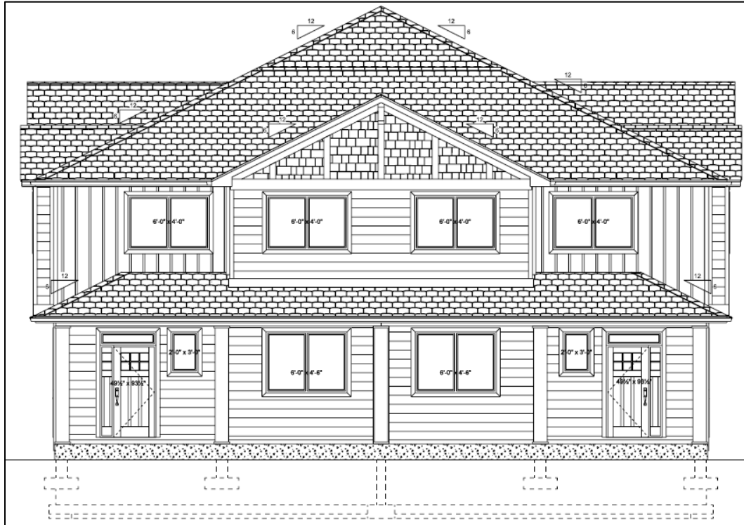
Figure 11: Rear elevation of duplex (from the lane)
