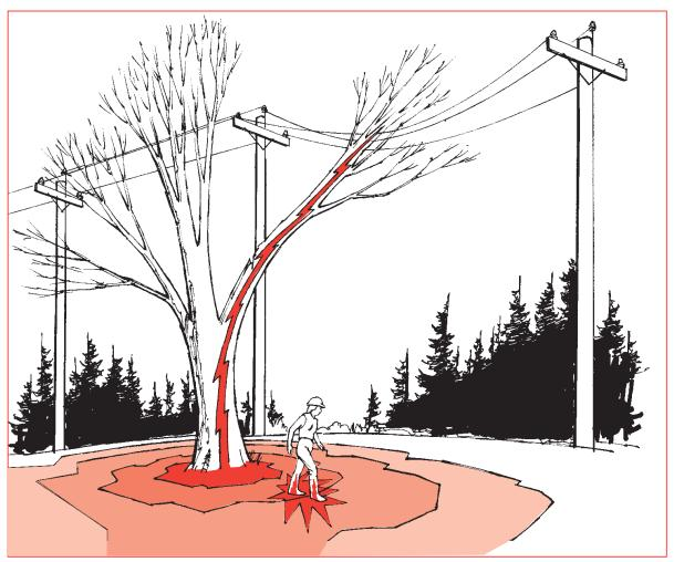
Step potential: If your feet are spread apart on energized ground, electricity can flow through your body from the area of higher voltage to the area of lower voltage.
