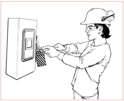
Apply a lock to the electrical disconnect switches before working on the equipment.
