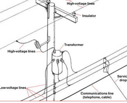
rhead electrical conductors can often be identified by their placement he pole.
