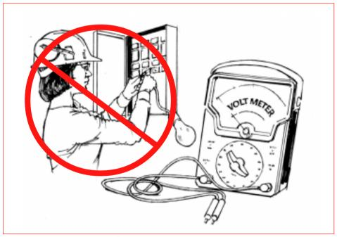
Use approved portable meters and leads, not an improvised test lamp.
