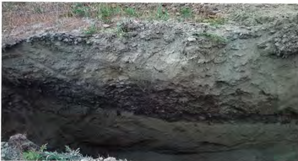
Figure 5. Pit M4 with a buried layer of crushed road asphalt starting at 40 cm.
