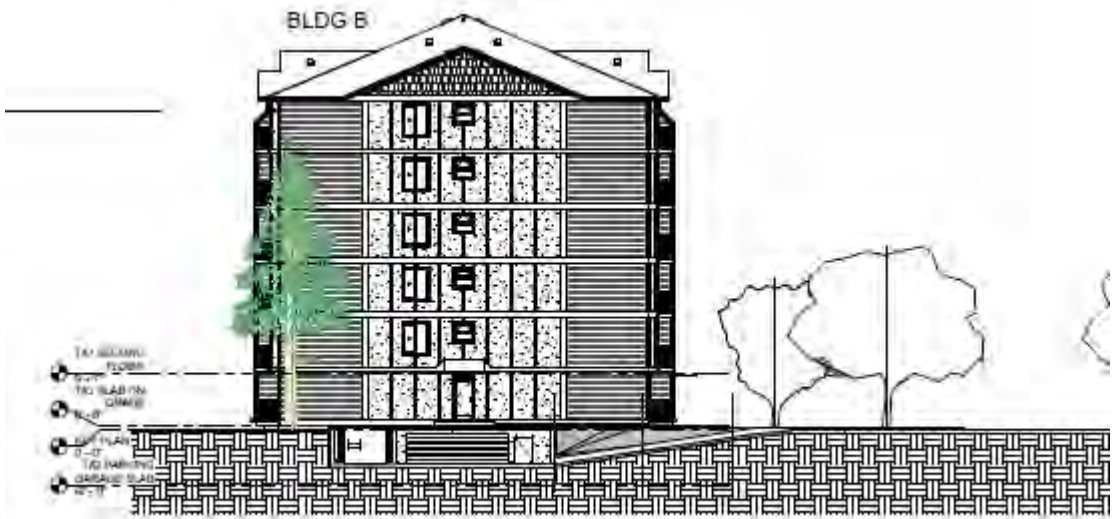
Figure 12: Right Elevation ( showing underground parking)
