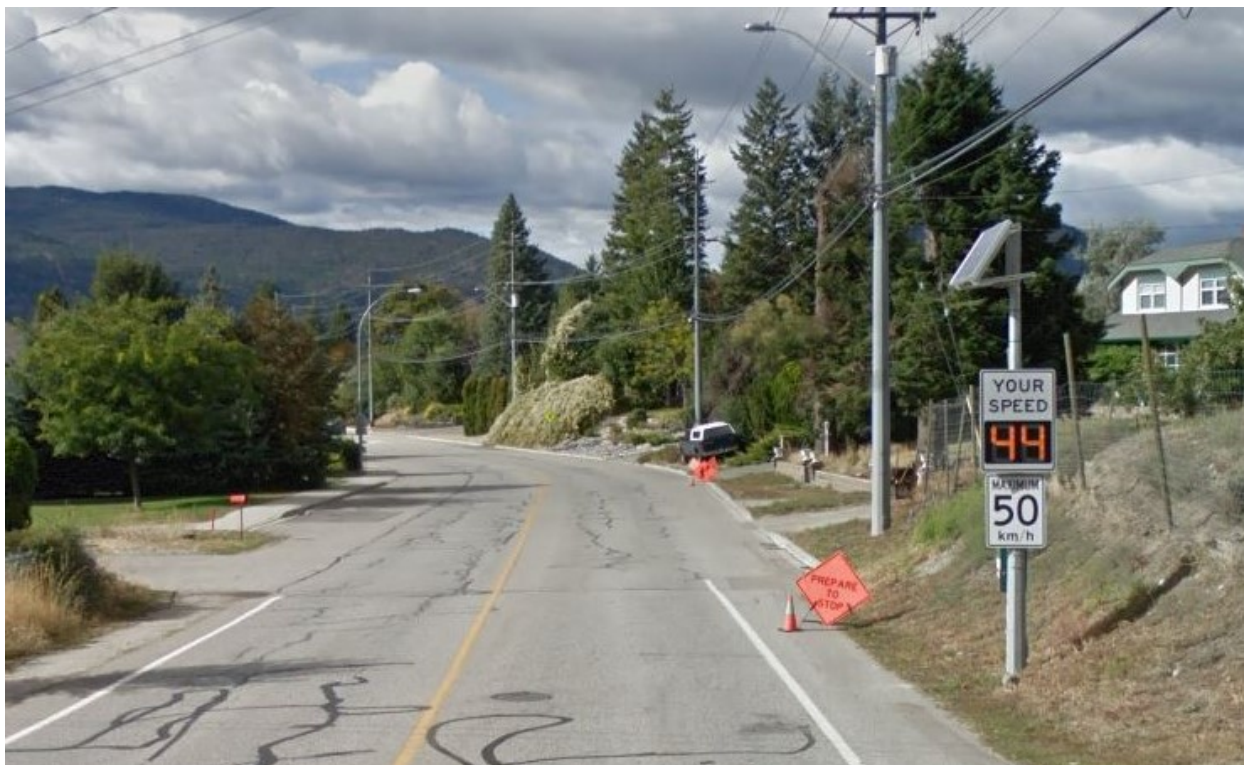
Figure 1 – Solar Powered Post Mounted Driver Feedback Sign Installed on Johnson Rd (2011)
