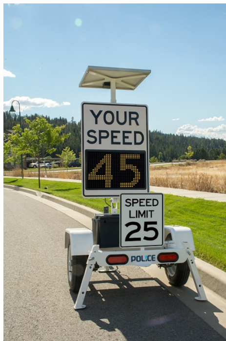
Figure 2 – Solar Powered Driver Feedback Sign – trailer mounted
