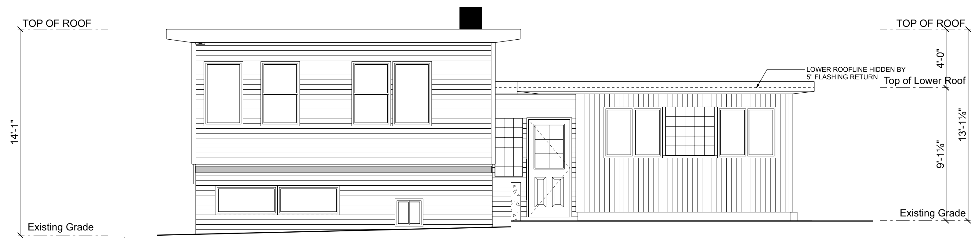
HOUSE FRONT ELEVATION (FACING FORESTBROOK DR.) SCALE: 1/4" = 1'-0"
