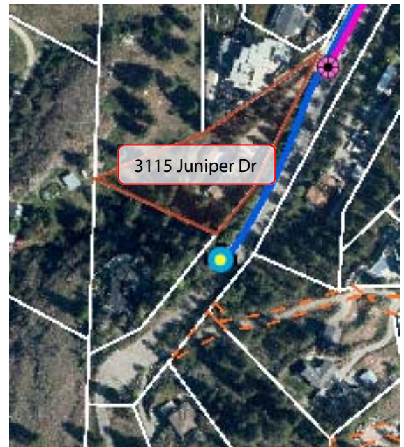
Figure 2 - Extent of municipal water main (blue) and municipal sanitary sewer main (pink) in Juniper Drive. Both services will be extended to the cul-de-sac by a different developer.
