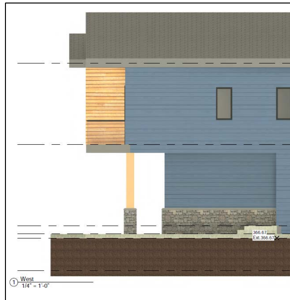
Figure 4 - Side view of proposed cantilever over driveways
