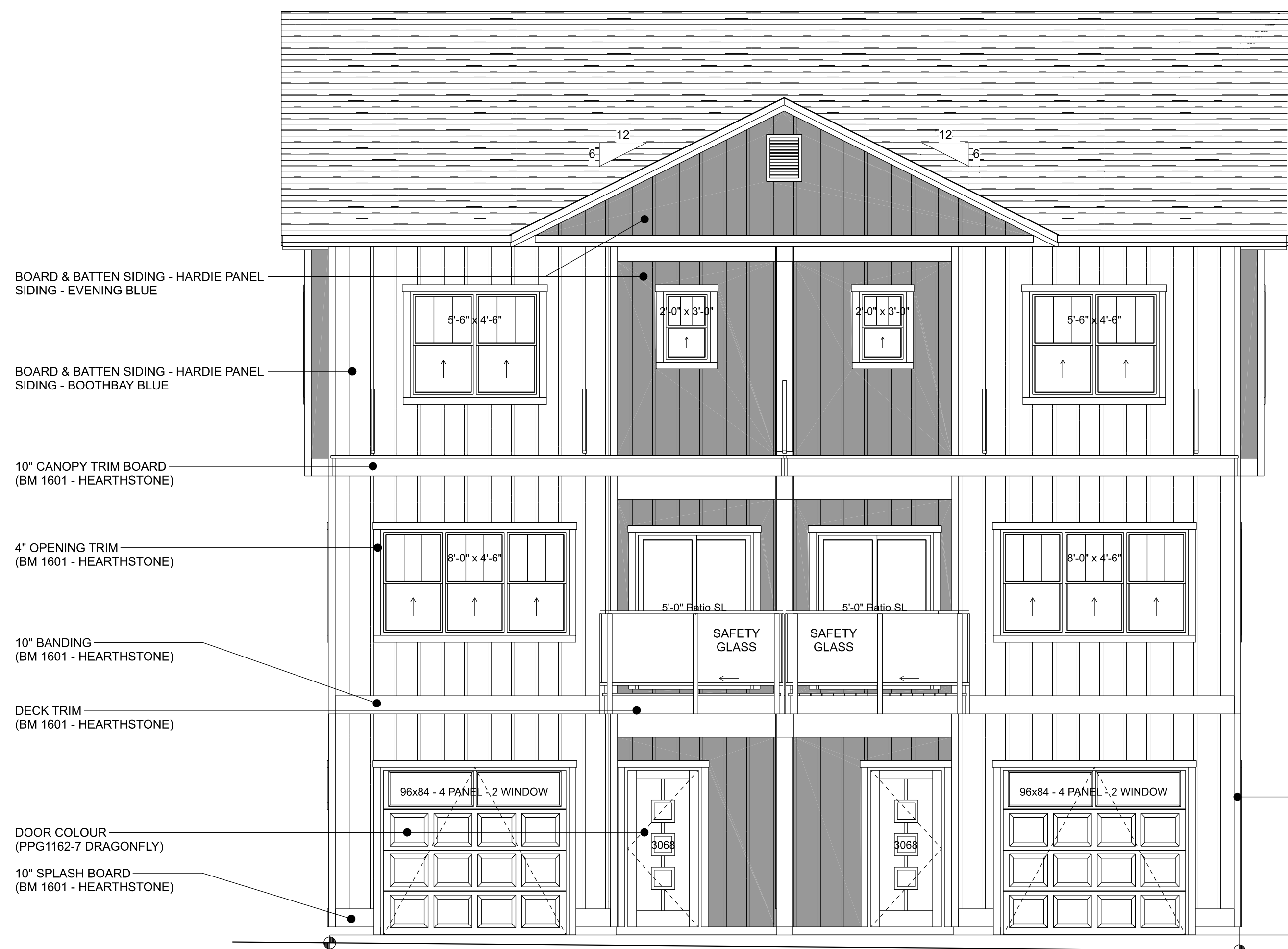
NORTH ELEVATION - BUILDING B SCALE: 1/4" = 1'-0"
