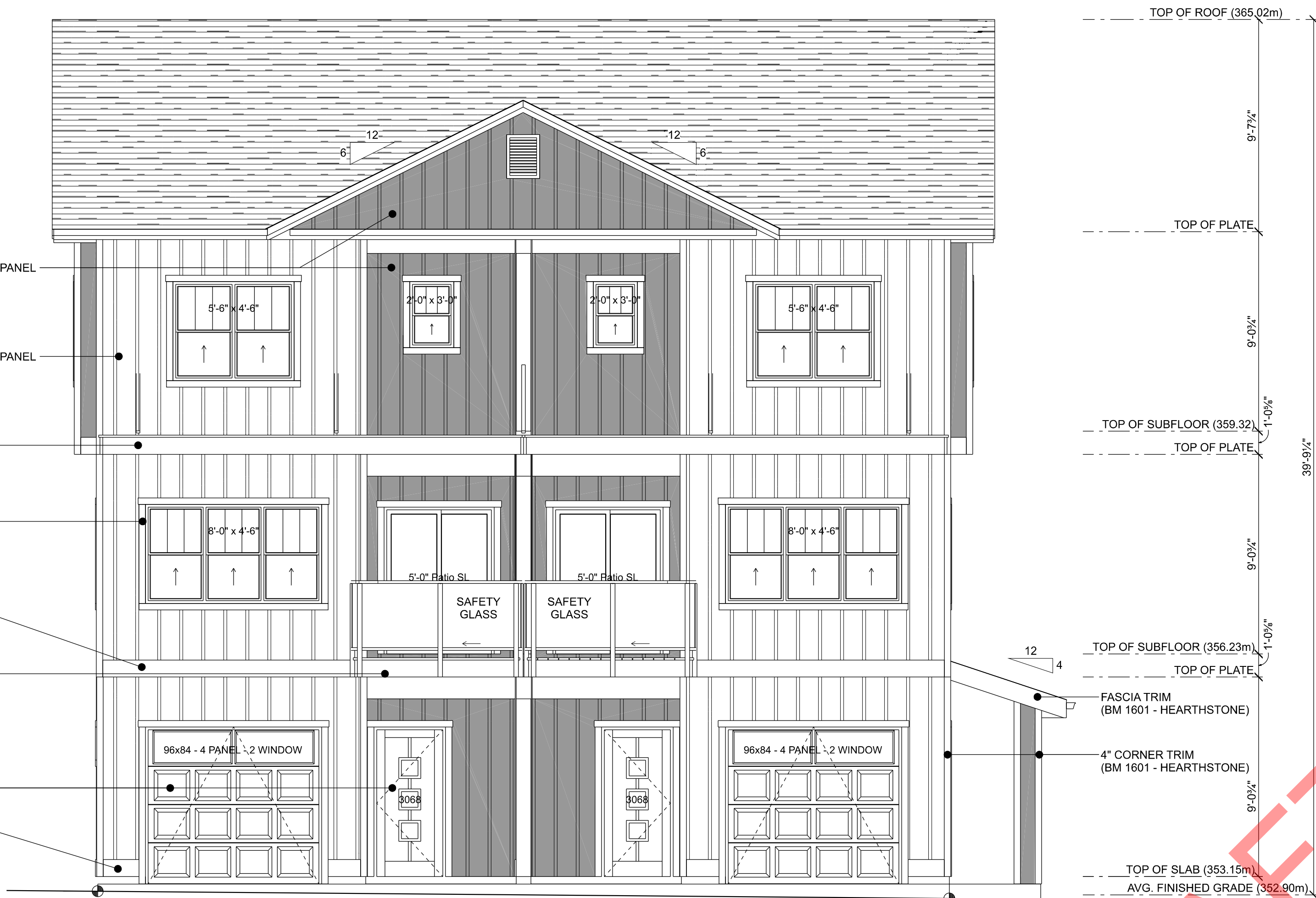
NORTH ELEVATION - BUILDING A SCALE: 1/4" = 1'-0"
