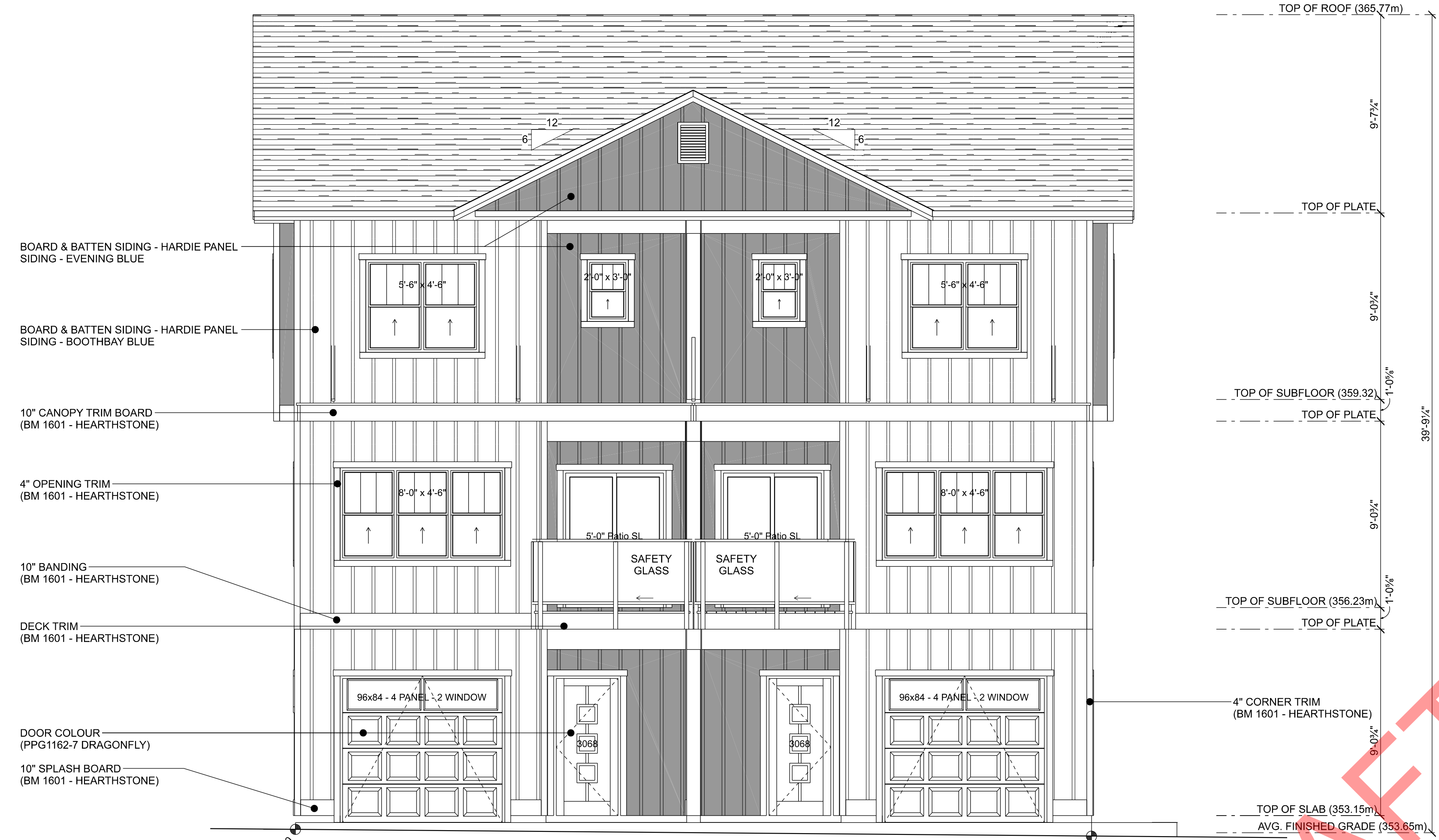
NORTH ELEVATION - BUILDING E SCALE: 1/4" = 1'-0"
