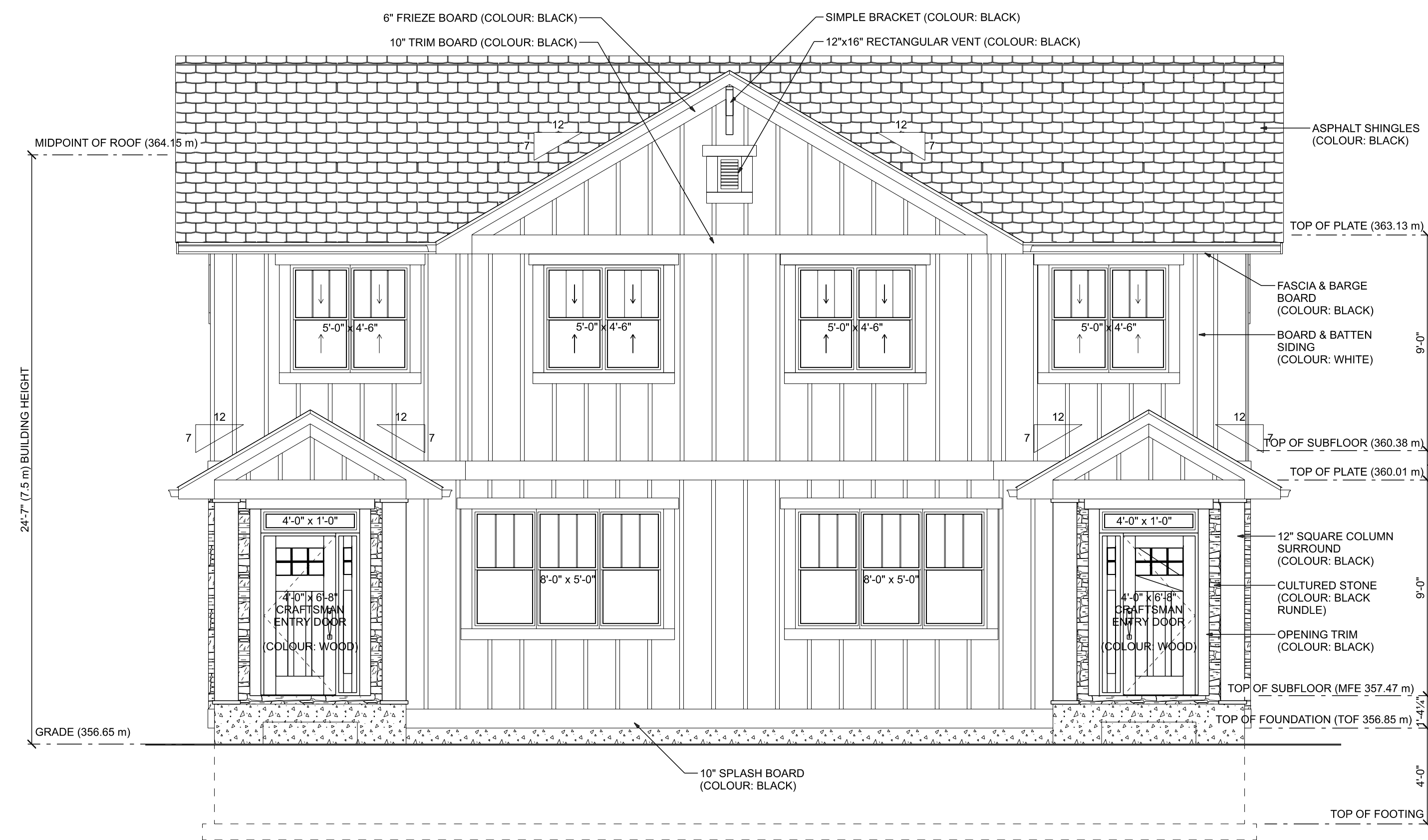
FRONT ELEVATION (TYPICAL BUILDINGS A & B) SCALE: 1/4" = 1'-0"
